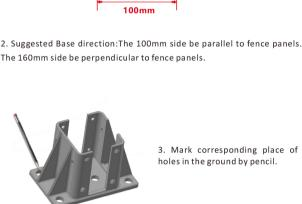
drill 4 holes Diameter: 12mm Depth: 60mm
