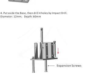
5. Fix the Base by Expansion Screws.
