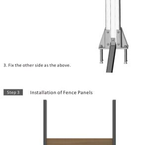
2. Put Rail into Post groove and fix it by Electric Drill and Drilling Screws.
